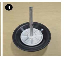
• The shaft (item 32) and shaft o-rings (item 30) should retain the lubricant that was factory applied. If they appear dry, apply a light coat of lithium thickened grease. Avoid over-lubrication as it can cause decreased performance of the air distribution system.
