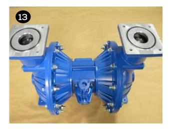
Stand the pump upright onto the suction manifold feet. Place the valve seat o-rings (item 13) into both sides of the valve seat. Place the seat on the liquid chamber (item 18). Place the valve balls (item 15) on the seats and discharge manifold (item 39) atop the components that are stacked on top of the liquid chambers. Install, tighten and torque the (8) manifold bolts (item 11).
