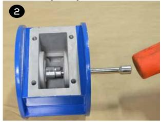
• Insert both bushings into the center section. Ensure the bushing is fully installed and the large rib on the outside of the bushing is flat against the center section.
