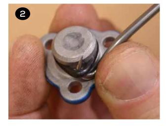
Remove the valve body (item 3) by removing the (4) socket head cap screws and washers (items 1 & 2) that attach the valve body to the muffler plate (item 38) with a 6 mm hex wrench Pull the valve body and gasket (items 3 & 36) off the front of the center section (item 35) and the muffler plate gasket, muffler plate and muffler (items 37, 38, & 40) off the back.
