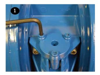
Plastic Air Valve - Remove and replace o-ring (item 5). Install cap (item 6) and tighten until groove for the retaining ring is visible. Install retaining ring.
