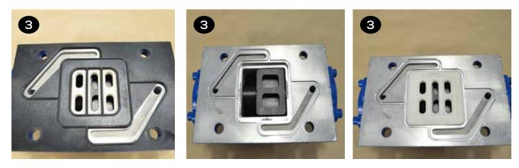
Insert the (4) cap screws & washers (items 1 & 2) through the valve body and gasket (items 3 & 36) and place onto the center section (item 35). Ensure the slide valve and valve plate (items 9 & 10) are in place and the valve sits flat on the center section.
