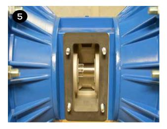
• Tighten and torque the (4) cap screws & washers (items 1 & 2) into the muffler plate.
