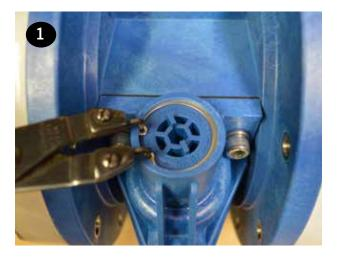
**Aluminum Air Valve** - To replace the valve cap o-rings (item 5), remove the (3) button head cap screws (item 7) using a 5 mm hex wrench.
