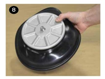
**9** The other diaphragm(s) (items 21/22) and inner/outer plates (items 19 & 23) can be installed onto the opposite end of the shaft (item 32).
